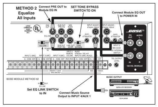
Fig. 26B - Method 2 Module Wiring Diagram
